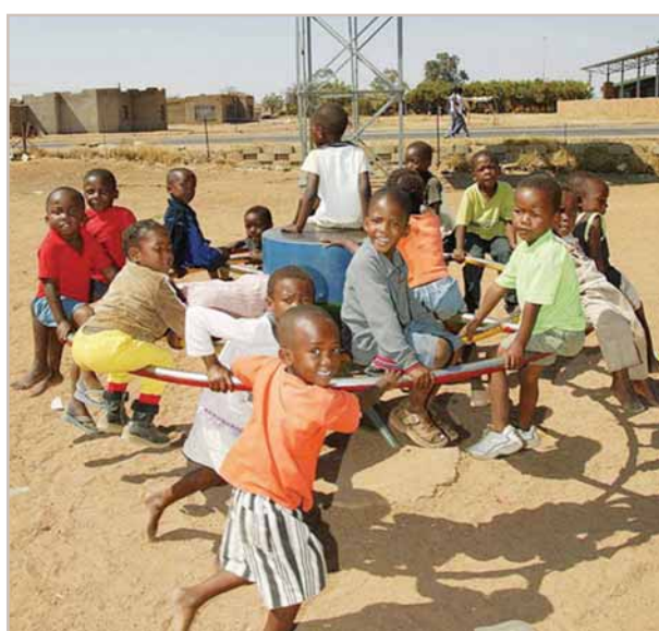
Using PlayPumps, kids pump clean water for a village while they play.
